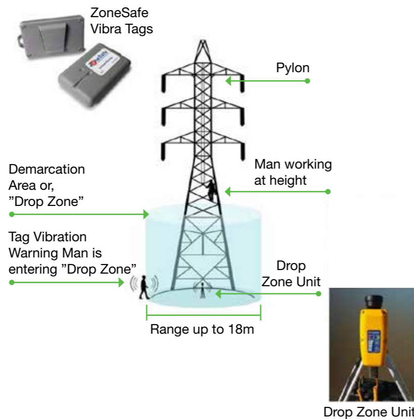
Drop Zone Unit
