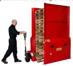
The PALOMAT® Flexomatic operates on compressed air and requires electricity for control of the machine.
