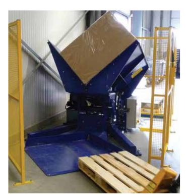
It will handle any conventional sized pallet with bottom boards and will transfer loads ranging from 60cm to 205cm in height.
