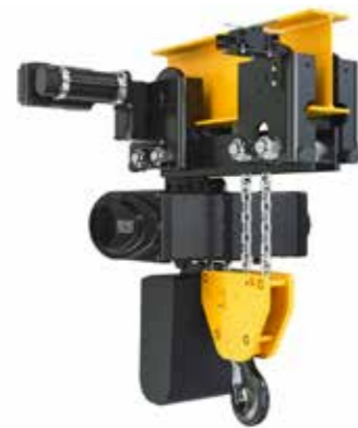
3 falls hoist body for increased capacity up to 7,500 kg coupled to motorized trolley on I beam.
