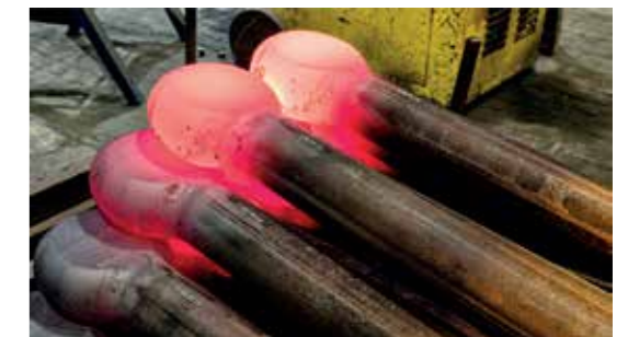
Zero-waste forging process: eyes are upset forged
